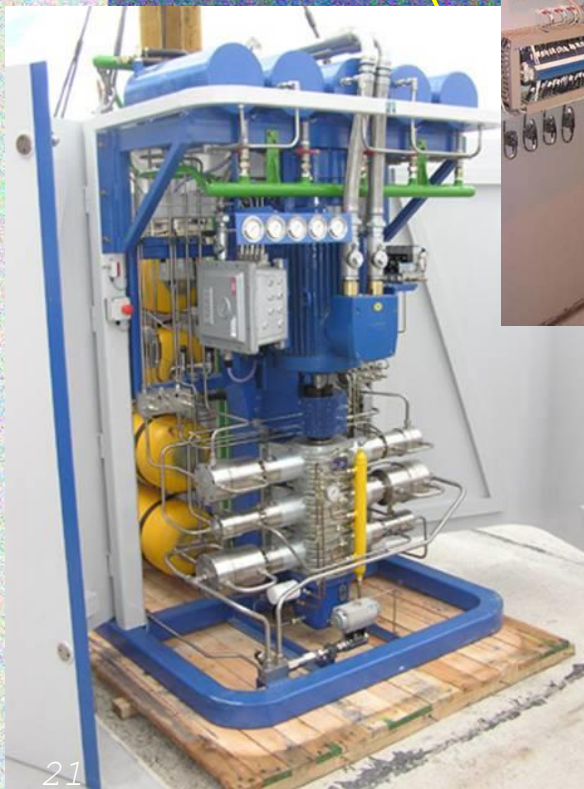
H2- Compressor & Storage Tanks
